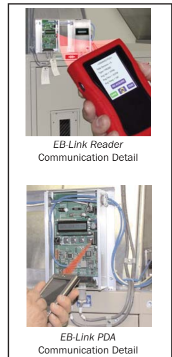
Figure 14. Typical EB-Link Data Acquisition
